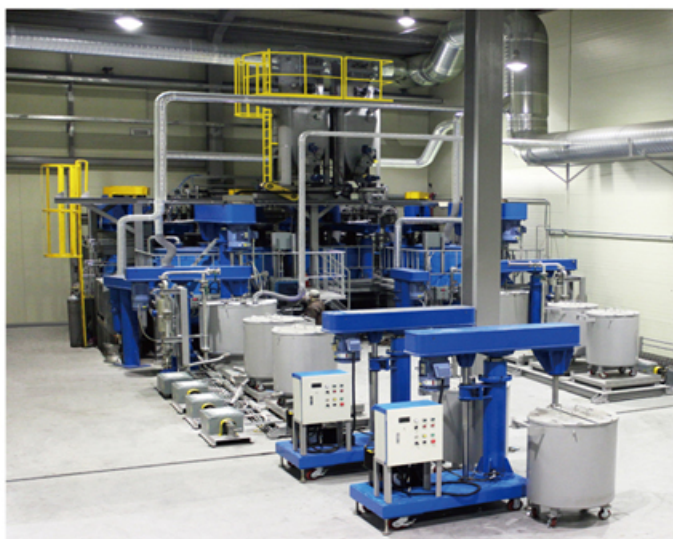
GRP (Raw Material) Stirring Line
